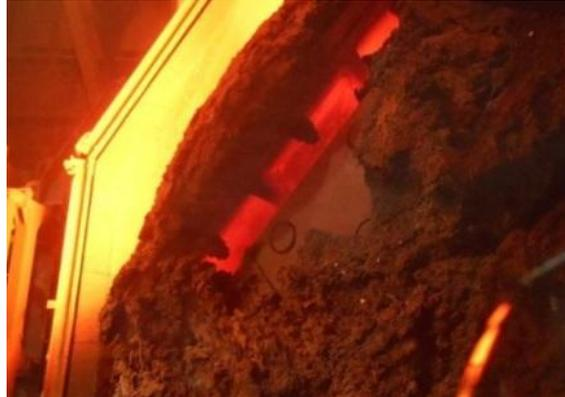
Fig. 7: Hot Spot in the Mouth Area Due to Post-Combustion Source: voestalpine
