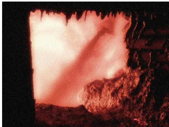
Figure 1. Injection of Carbonaceous Material into EAF using Straight Pipe Method
